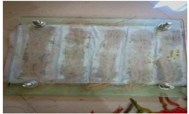
Fig.1 Hand Lap Up Technique for Composite
